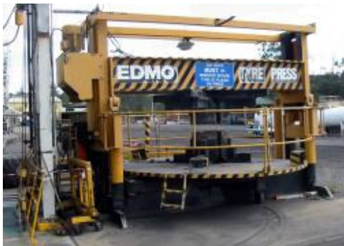
Photograph 01 left: Large Earthmover Tyre Press. Photograph 02 below: Fit for purpose bead-breaking tooling.
