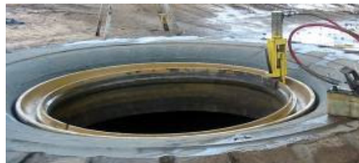
Photograph 01 left: Large Earthmover Tyre Press. Photograph 02 below: Fit for purpose bead-breaking tooling.
